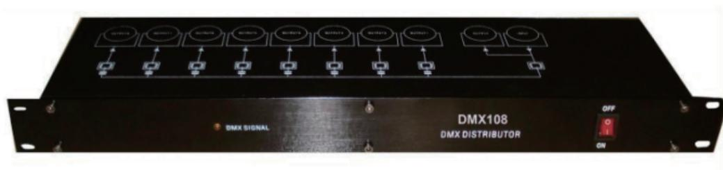
DMX-8(or DMX-4) Splitter is a DMX512 distribution amplifier It is specially designed for connection of DMX receivers (dimmers, color changers, moving lights,etc.) in a star configuration.
