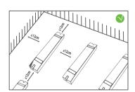
Please do not stack the products. The distance between two products should be>12cm so as not to affect heat dissipation and the lifespan of the products.
