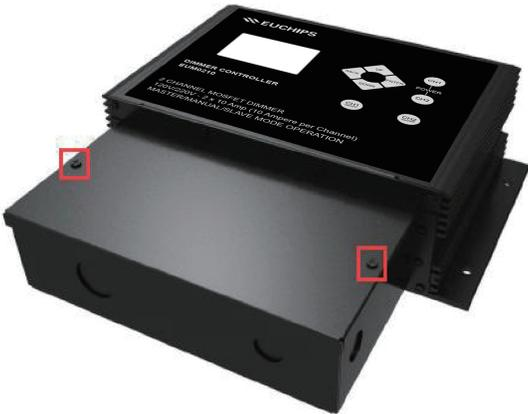
Knock-outs can be removed easily by pressing the round mark to connect Conduit of either "1/2" or "3/4" inch size. Remove the screws from the sides to remove electrical cover as per need.
